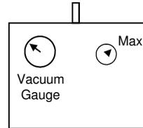
Disconnect all items from inlet and with pump switched off, confirm that gauge reads zero. A non-zero reading indicates a faulty gauge.
