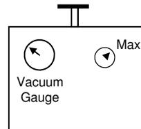
Switch on pump and occlude inlet. Note maximum vacuum reading.
