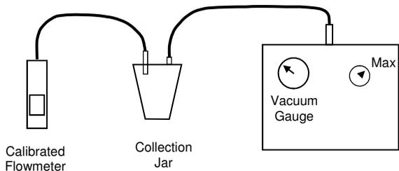
Connect pump as shown in diagram. Set vacuum control knob to maximum, and switch on pump. Connect jar inlet to calibrated flow meter and note flow reading. If flow is significantly below specification, check internal tubing and pump itself (or internal shutoff valve if fitted).
