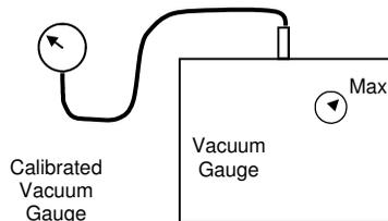
Connect a calibrated vacuum gauge directly to inlet and repeat maximum vacuum reading.
