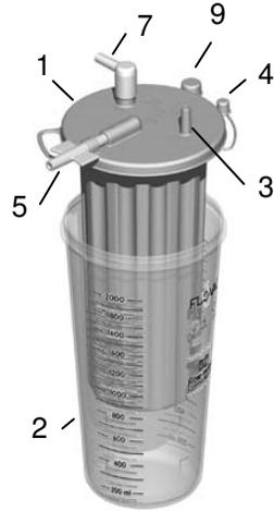
Note: For disposable jars only, which have an antibacterial filter built-in to the lid, connection may be made directly to the pump inlet nipple.
