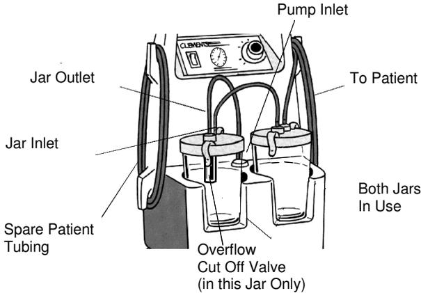
To connect the Collection Jars in a double-jar arrangement, use the following procedure and refer to the block diagram below.
