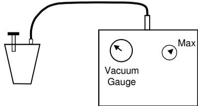
Connect pump as shown in diagram. Set vacuum control knob to maximum, and switch on pump. Occlude jar inlet and confirm that pump achieves the same maximum vacuum as in the previous vacuum check setup. Any difference indicates leaks in jar or connections.
